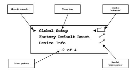
The currently selected menu item is enclosed on the left and on the right by the menu item marker. Use keys **up** and **down** on the front panel to move the menu item marker to the desired menu item. To select a menu item press key **set** shortly.
