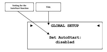
Press the key **up** on the front panel to activate the AutoStart function. If you like to disable the AutoStart function press the key **down**.
