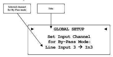
Use keys **up** and **down** on the front panel to select the input channel you would like to use in By-Pass Mode.
