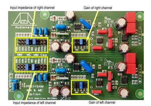
For each channel several jumper fields are available for setting up input impedance and gain.
