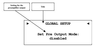
Press keys **up** on the front panel to activate the preamplifier output **PRE OUT** 16. If you like to disable the preamplifier output press key **down**.
