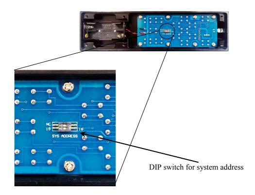
Put the DIP switch labelled 'SYS ADDRESS' in position '19' or '16' according to the following table:
