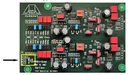
(2x100p for SAM is printed on the PCB right beside the capacitors)
