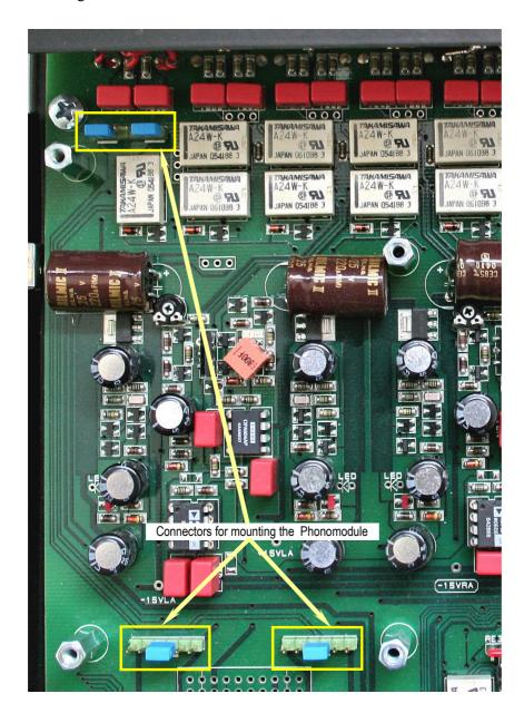
Remove all 4 jumpers on the 3 connectors. Push the Phonomodule with its 3 jacks on the bottom side onto the 3 connectors until the module sits tight on the mounting bolts. The orientation of the module is determined by the alignment of the connectors.
