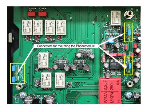
Remove all 4 jumpers on the 3 connectors. Push the Phonomodule with its 3 jacks on its bottom side onto the 3 connectors of the MAP 1 /
