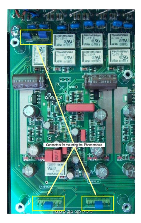
Remove all 4 jumpers on the 3 connectors. Push the Phonomodule with its 3 jacks on the bottom side onto the 3 connectors until the module sits
