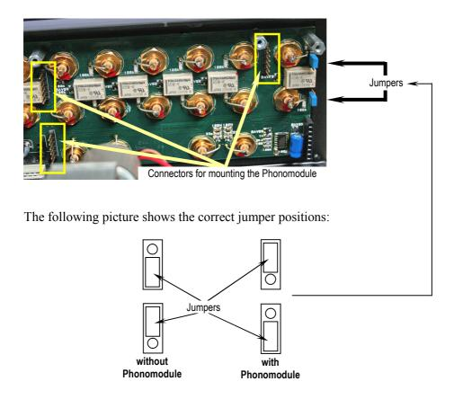
Push the Phonomodule with its 3 jacks on the bottom side onto the 3 connectors on the input board marked in the picture above until the module sits tight on the mounting bolts. The orientation of the module is determined by the alignment of the connectors.
