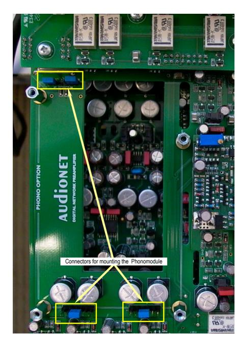
Remove all 4 jumpers on the 3 connectors. Push the Phonomodule with its 3 jacks on the bottom side onto the 3 connectors until the module sits tight on the mounting bolts. The orientation of the module is determined by the alignment of the connectors.
